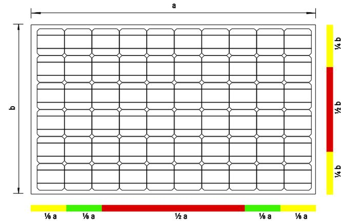
A minimum of four clamps must be fully located in the same colored zone to be certified to that value. If the panel is secured by four clamps in two different zones (i.e. green and yellow), it is certified to the lowest value only.
